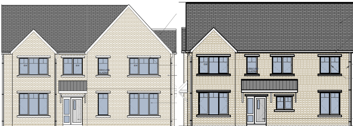
Figure 56.0 Front elevation of House Types A and AD (left) and side elevations of House Types A and AD illustrating entrance to House Type AD (right).
